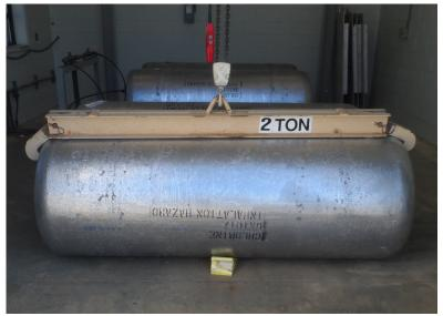
• Once the containers or cylinders are unloaded, secure them properly at the site. Always store cylinders in an upright position. Store ton containers with the two valves lined up vertically.
